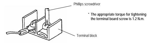
Figure 5.6 Connecting a Cable to Terminal Block
